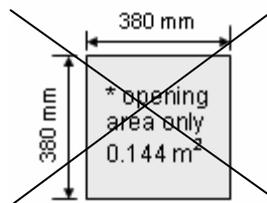
The opening in example A is only  $0.144 \text{ m}^2$ , and it will not allow the average occupant to pass through the window as an alternate means of escape during a fire emergency.
